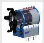
ARRI's cross cooling system moves a stream of air around the Fresnel lens and through the lamphead. In addition, air is channeled through the aluminium extrusion housing reducing lens temperature by 17 % and housing temperatures by 25 %. Cross cooling allows ARRI True Blue fixtures to safely operate at almost any tilt angle.
