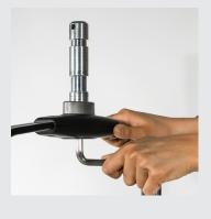
Before mounting the fixture, attach the proper mounting hardware to the stirrup. A spigot and flange\* is included inside the box and should be attached with a 10 mm hex or Allen key. The bolt must be fully tightened (50 Nm of torque are adequate).
